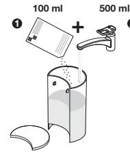
③ Empty the drip tray, drip base and capsule container. Fill the water tank with 500 ml of fresh drinking water. Pour 1 pouch of *Nespresso* liquid descaling agent into the water tank.
