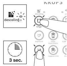
**6** To enter the descaling mode, simultaneously press the Lungo + Ristretto keys for 3 seconds. Both keys blink. To start the descaling program press the same keys again.
